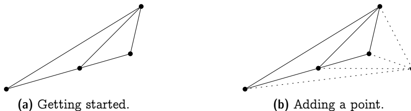
Figure 5.2: Constructing the scan triangulation of P .
