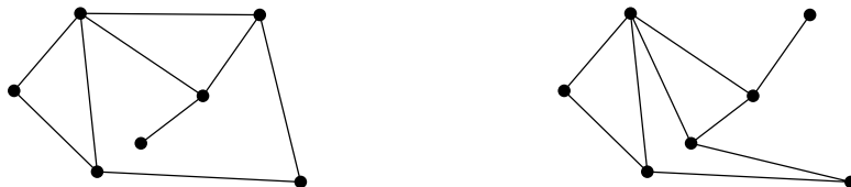
Figure 2.6: An outerplanar graph (left) and a plane embedding of it in which all vertices are incident to the outer face (right).
